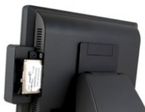
Slide in/out HDD Replacement
